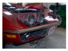
hose kit was available aftermarket, so out with the old washer hose and in with the new. Replacing the metal tube along the left hand wiper arm along with the new hose and clamps was yet another story. In order to get at it, I had to remove not only the wiper grill, but the entire wiper door....believe me having fat fingers is not an advantage here!
