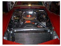
did this in part because last spring, I had just replaced the condenser and had converted the A/C system form R12 to R134 and I didn't want to open the system back up.
