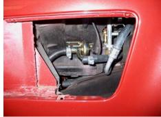
While in the engine compartment, I also replaced the horn/key buzzer relay with the correct case markings. Ditto for the high speed blower relay mounted on the passenger side firewall.
